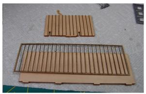
Taking full advantage of the laser cutter capabilities, Bar Mills uses a two step process -- a blank wall underneath, and a veneer overlay that carries the battens in place until placed on the under wall. This can be a little confusing at first -- as the photo at left demonstrates, the battens are attached to an exterior frame, the entire unit is placed on the under wall, and then the outside carrier pieces are removed.
