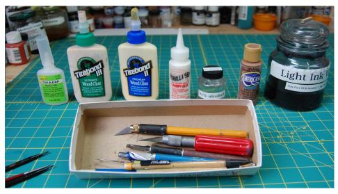
I use Titebond instead of white glue because Titebond is NOT water soluble, and we use some water in weathering. The light ink is in an old candle jar, which has a terrific seal. I wrote the recipe on the label for consistency of wash.
